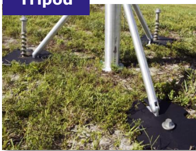
PE18 Temporary mount for solar panel to power equipment in the field
