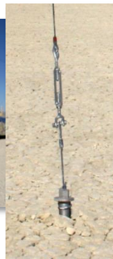
PE26 with tie-off cable to turnbuckle
