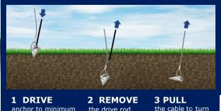
anchor to minimum depth of 21/21 (.8 m)
