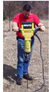
Demolition hammer or small jackhammer depending on soil conditions
